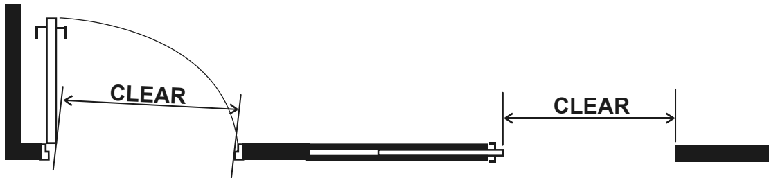
Figure 1. Clear Opening Measurement For Doors
